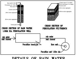
DETAILS OF RAIN WATER **HARVESTING STRUCTURES**
